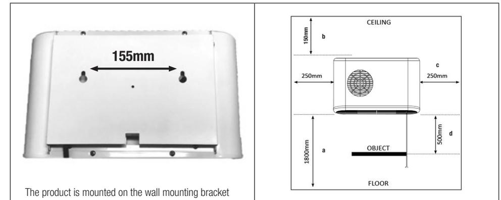
The product is mounted on the wall mounting bracket
