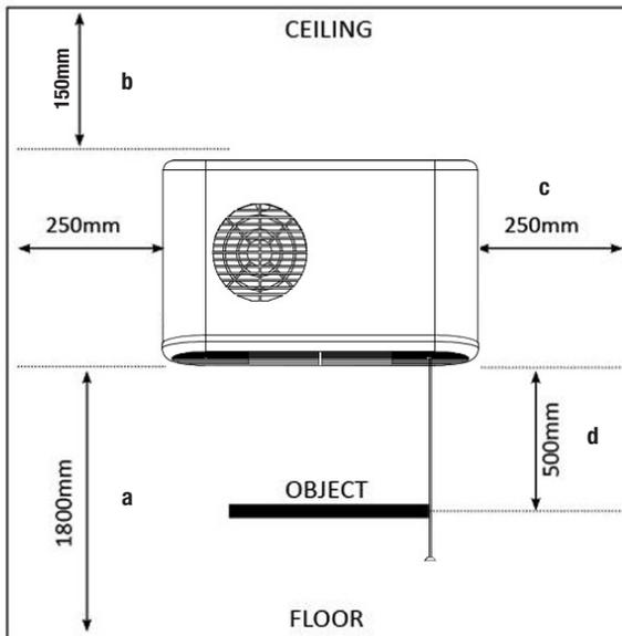
The air is sucked in, blown over heating elements and then blown out through the lower grille into the bathroom. The heater functions (On/Off, temperature adjustments) are controlled by the pull-cord switch.
